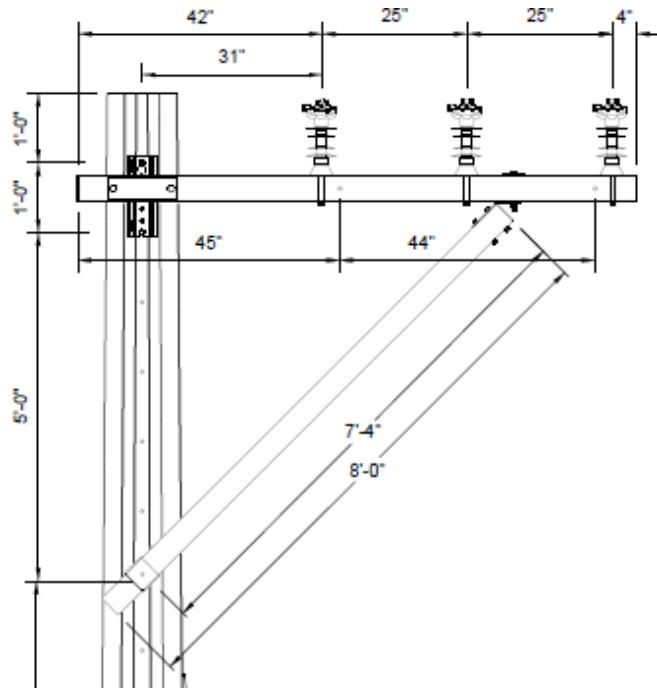
2. **Case 2:** As seen in the figure below, a hole shall be located 81 in. (6 ft.-9 in.) away from the center of the mounting bracket and 4 in. away from the end of the crossarm (unattached end).
