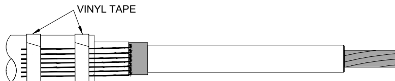
FIGURE G-1 JACKETED CONCENTRIC NEUTRAL (JCN) CABLE
