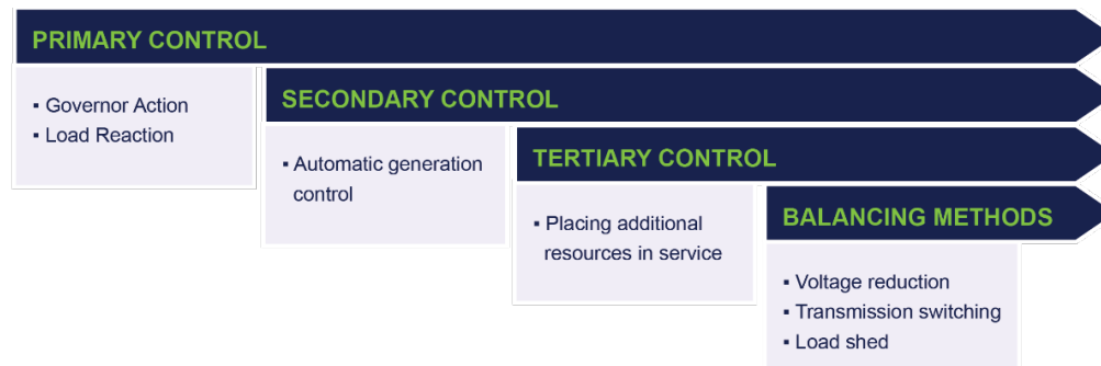
Figure 10-1. Typical hierarchy of control to maintain frequency and voltage
